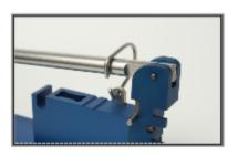
5. Spreads Rings: Make sure hub is completely removed with hub cutter. Slide tamperproof ring over handle with opening facing as shown in picture. Then hook lower end into the eyelet that protrudes up from the vice base. Place one hand on the front base plate of the vice while pulling up on the handle, spreading ring to desired opening.
