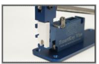
3. U-Ring Press: After cutting the u-ring from the SmartKey, you will need to remove the fragment of the u-ring left inside the SmartKey. To do this, place the SmartKey at the back of the SmartKey Vise with the notch facing left (as pictured). Align the hole on the SmartKey with the pin on the vice and slowly raise the lever. This will press the u-ring fragment into the SmartKey chamber, allowing use of another u-ring.
