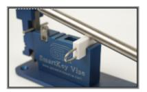
2. Secure SmartKey: Place your SmartKey with the notched side facing upwards in the slot and in line with the lever handle. (U-ring can be on the left or right side.) Apply pressure on the lever handle to firmly hold your SmartKey from moving. Using a small hacksaw or Dremel, cut the top side of the stainless steel u-ring, flush with the edge of the SmartKey. After cutting the top u-ring, remove the u-ring by pulling it out of the SmartKey and discarding it.
