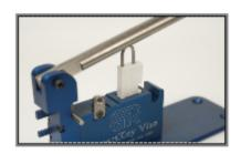
1. Seals SmartKeys: Place the SmartKey in the top chamber twards the center of the vise. Place the new u-ring in line with the holes in the top of the SmartKey. Make sure that the notched end of the u-ring is inserted in the hole on the same side as the notched side of the SmartKey. Bring the lever handle downwards to push the u-ring in.
